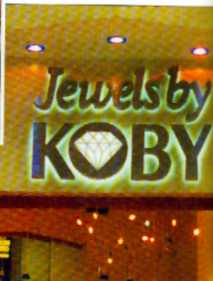
This is one of 10 stores that Gregory Signs supplies signage to. They are back lit, hand-bent letters. The diamond shape in the "O" was made by cutting out the center and replacing it with acrylic. The diamond cuts are vinyl.
